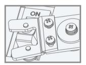
The push handle adopt adjustable slider structure design, have more wide circuit breaker's ON/OFF travelling distance, make the production process more simple.
